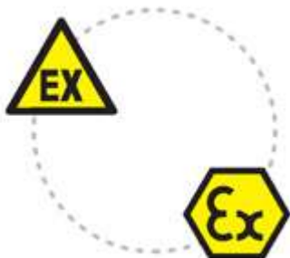
- Figure 2 Explosive area signage and material equipment designation.
